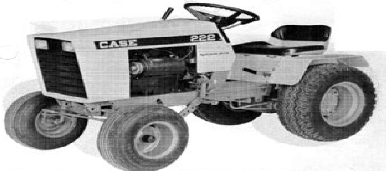
Figure 2. Left Hand View of Case 222 Tractor with Optional Hydraulic Lift
