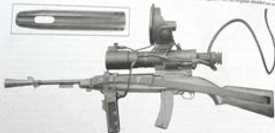
Fig. 9-7. An M2 Carbine with the M3 Sniperscope system mounted. The M3 was designed to be easily mounted on an M2 carbine using an extended Redfield-type mount that was secured at the rear of the receiver at the rear sight dovetail and extended forward to clamp around the barrel under the handguard. A single dovetail hole was drilled through the handguard for the clamp to attach to the barrel (note: M3 original original M3 Sniperscope have been mounted on M2 Carbines). Gordon Lambert collection.
