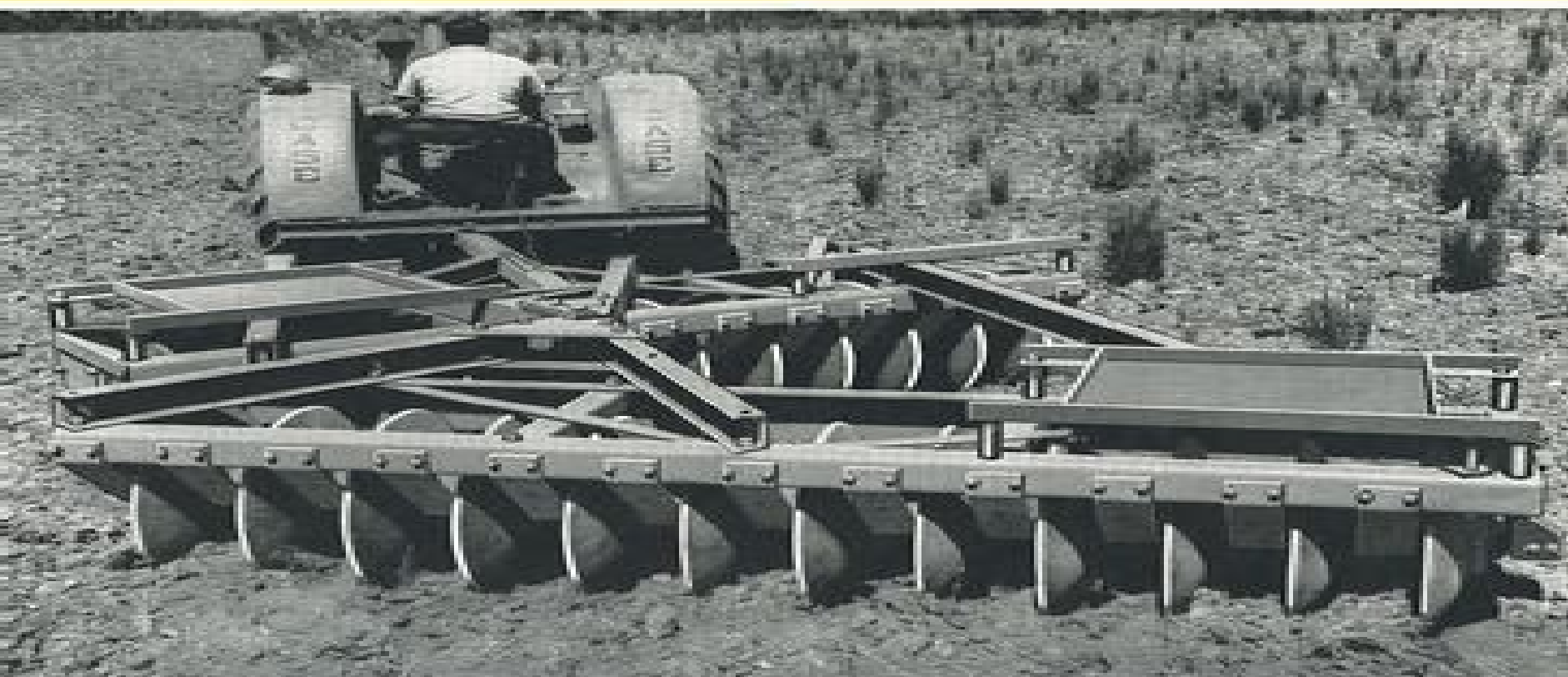
24 PLATE LITTLE GIANT WORKING FALLOW IN VICTORIA. 8 FEET CUT.
